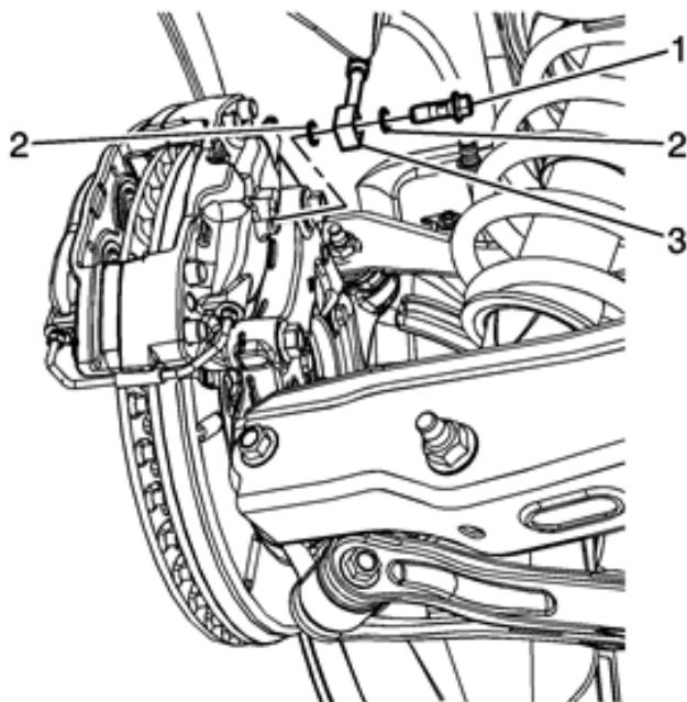
1. Remove the hose fitting bolt (1).
