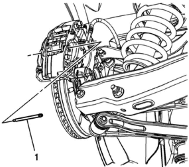
7. Hold the end of the brake pad spring down and carefully drive the lower brake pad pin (1) into the brake caliper.
