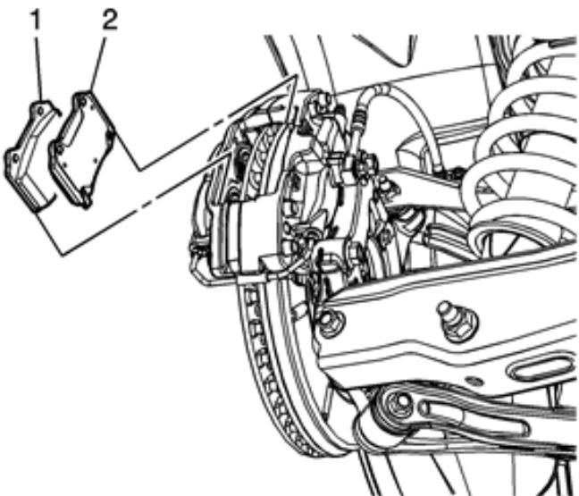
1. Install the outer brake pad (1).
