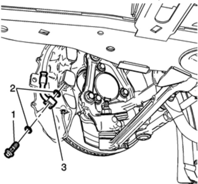
1. Assemble the brake hose fitting bolt (1) with 2 new brake hose fitting gaskets (2) to the brake hose (3).
