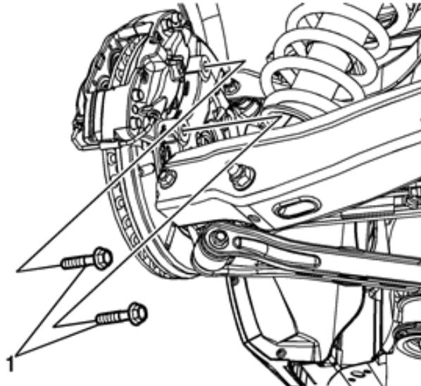
**NOTE:** The brake caliper bolts must be replaced.
