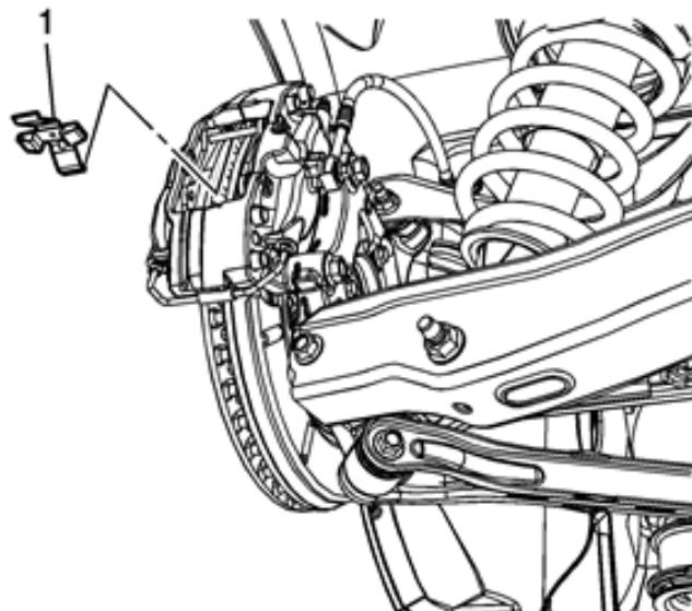
6. Install the brake pad spring (1).
