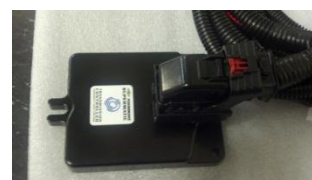
Transmission Control Unit Connection
