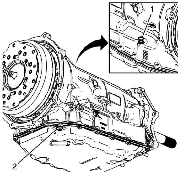
**Caution:** Use Dexron® HP transmission fluid only. Failure to use the proper fluid may result in transmission internal damage.
