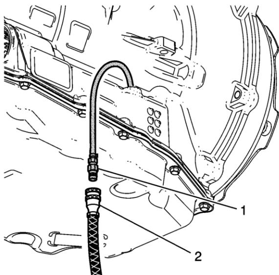
**Note:** The DT-45096 flush and flow test tool is being utilized as a convenient method to pump the fluid into the bottom pan. A suitable hand pump may also be used instead. When using the DT-45096 flush and flow test tool, monitor the display panel to determine the amount of fluid being pumped from the tool supply tank into the transmission.
