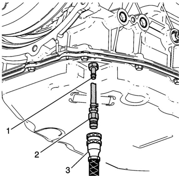
2. Install the DT-51190 fluid fill pan adapter (1) and, if necessary, one adapter from the DT 45096-30 cooler flush adapters (2).
