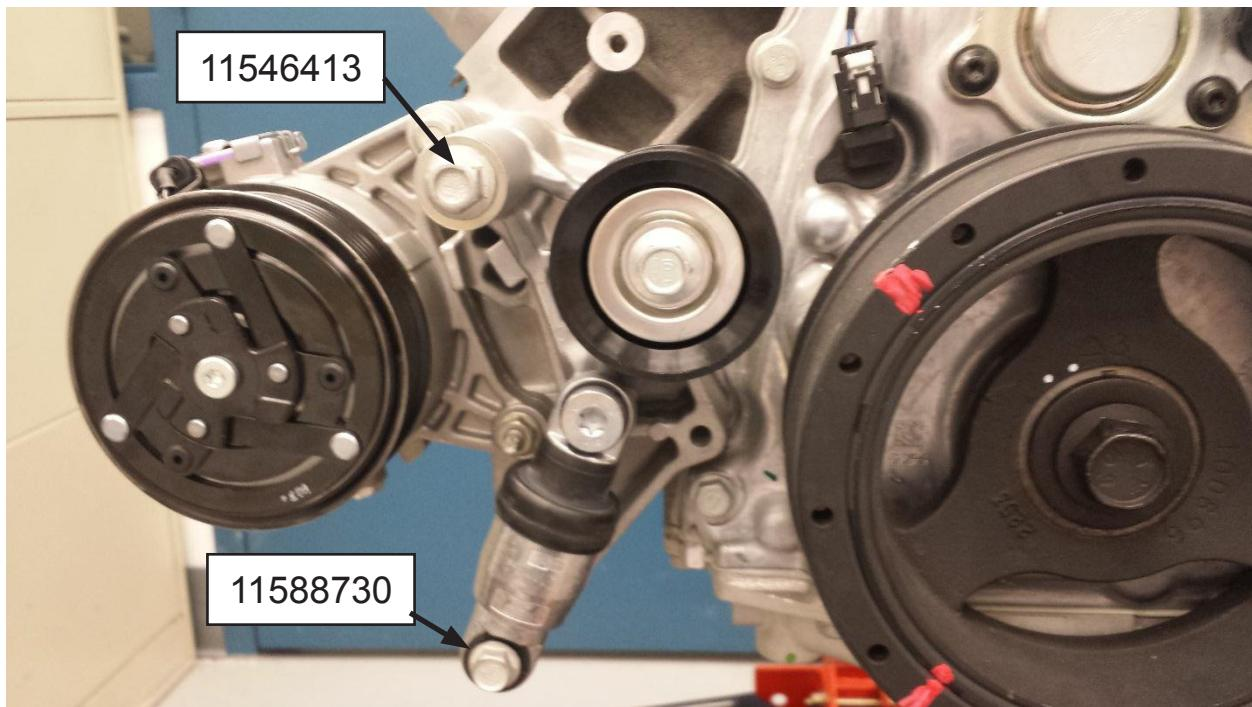
4. Install generator using (2) 11546413 bolts. Torque to 54 NM (43 lb ft).
