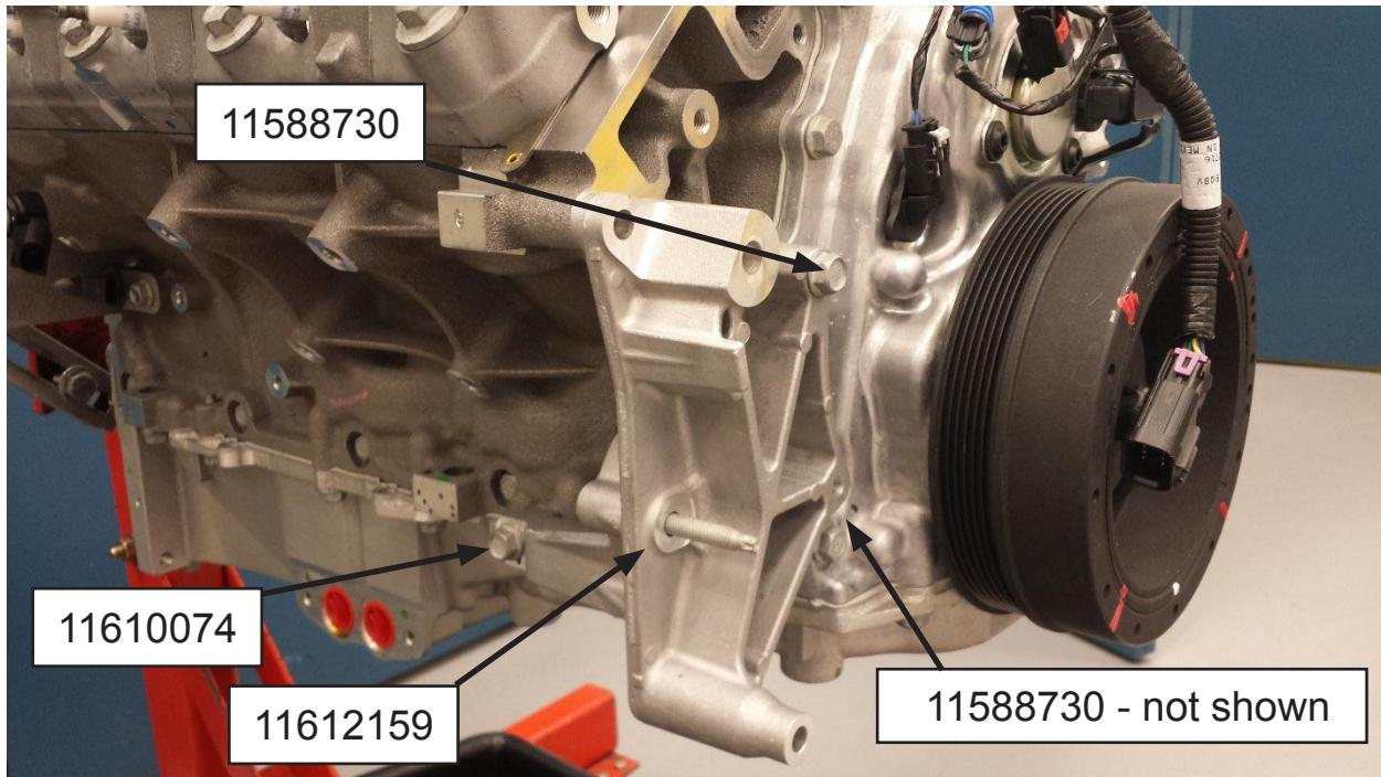
2. Install A/C Compressor 23105946 using 11588694. Torque to 22 Nm (16 lb ft). Install nut 11610074 on stud. Torque to 22 Nm (16 lb ft).
