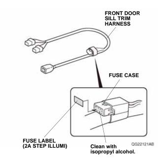
27. Plug the vehicle 2-pin connector into the front door sill trim harness 2-pin connector, and secure the 2-pin connectors to the vehicle harness with one wire tie.
