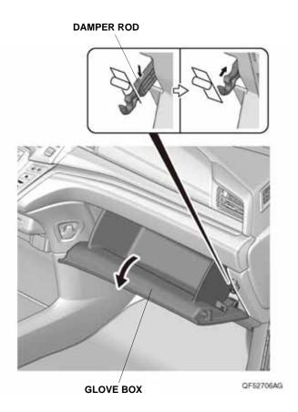
4. Close the glove box, and remove the two bolts from the glove box.
