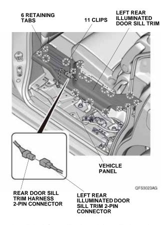
40. Install the left rear illuminated door sill trim to the vehicle panel.
