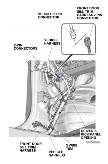
20. Route the front door sill trim harness along the vehicle harness, and secure it to the vehicle harness with two wire ties.
