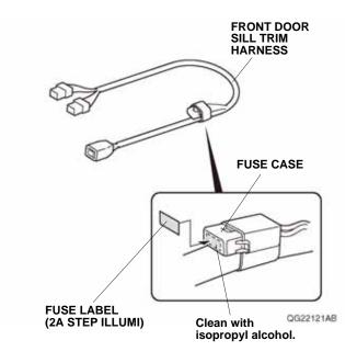
Plug the vehicle 2-pin connector into the front door sill trim harness 2-pin connector, and secure the 2pin connectors to the vehicle harness with one wire tie.
