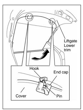
3. Slowly pull out the cover and secure the cover ends (end cap pins) into the liftgate lower trim retainers (2 locations).
