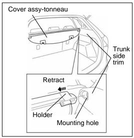
2. Retract the holder on the right end of the cover assy-tonneau and insert it into the mounting hole.
