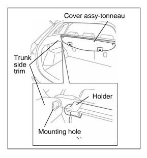
1. Insert the holder on the left end of the cover assy-tonneau into the mounting hole of the trunk side trim.
