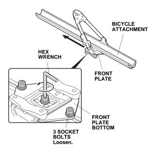
Set the front plate 245 mm (9.6 in.) from the end of the bicycle attachment, and retighten the three socket bolts on the bottom. Torque the three socket bolts to 8 N·m (5.9 lbf·ft). Rotate the arm as shown.
